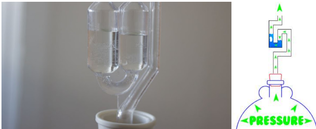
Figuur 1: A picture (left) and schematic (right) of a fermentation or air lock. Source: https://www.howtohomebrewbeers.com/ and https://www.stonehelm.co.uk/
